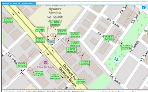
Load Flow calculation results with geographical map
