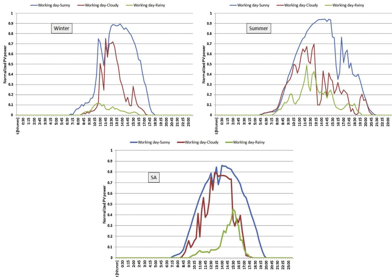
Fig. 10. Normalized PV generation profile for working days in winter, summer, and SA.
