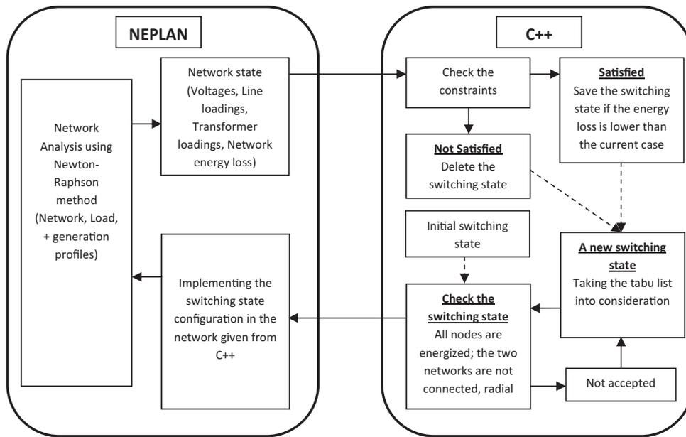
Fig. 2. Interaction between NEPLAN and C++.
