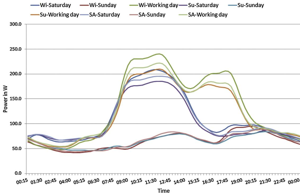
Fig. 6. VDEW load profiles of commercials (G0).
