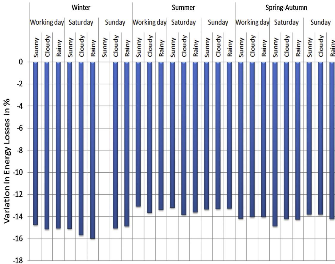
Fig. 11. Variation in the energy losses for different investigated days.
