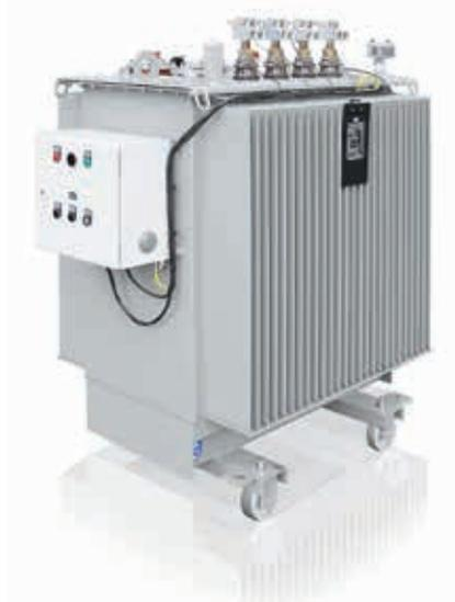
Based on these conclusions, ABB developed a voltage-controlled distribution transformer known as Smart-R Trafo<sup>2</sup> to match the requirements of distribution system operators → 3. It is based on an economic on-load tap changer that changes voltage in five steps and provides adequate power quality for distribution grids. Smart-R Trafo is expected to become a standard asset for distribution grid operators in Germany and other markets.
