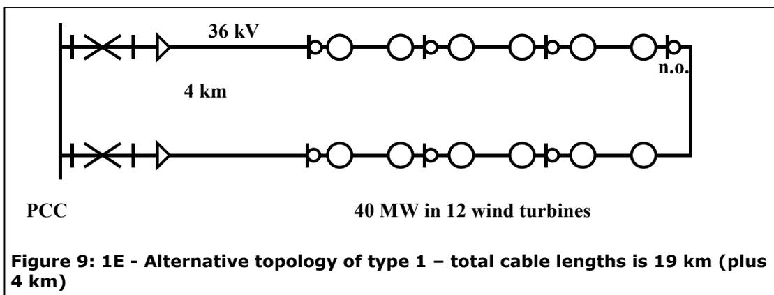
Alternative topology 1E is topology 1D with more load-switches. The redundancy consist of an additional feeder cable capable of 40 MW, an additional switchgear in the PCC, seven wind turbine-placed load-switches and control system. The system is radial and both feeder cables can transfer 40 MW each. The expected annual energy not supplied for this system is **4.146 GWh** (350 GWh).
