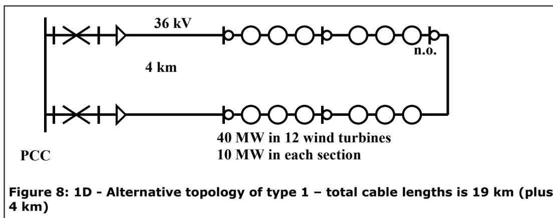
Alternative topology 1D, with double feeder cables, a normally opened cable loop and load-switches. The redundancy consist of an additional feeder cable, an additional switchgear in the PCC, three wind turbine-placed load-switches and control system. The system is radial and both feeder cables can transfer 40 MW each. The study shows an expected annual energy not supplied of **4.491 GWh** (350 GWh).
