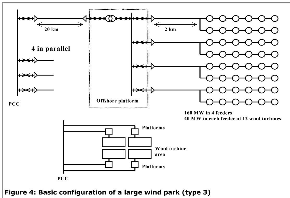
**Figure 4: Basic configuration of a large wind park (type 3)**
