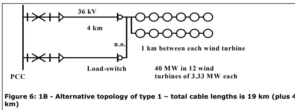
Alternative topology 1B, where an additional feeder is used. The redundancy consist of an additional feeder cable, an additional circuit-breaker in the PCC, two wind turbine-placed load-switches and remote-control system. The expected annual energy not supplied is **9.324 GWh** (350 GWh). The main contribution is from all the interconnecting wind turbine cables.
