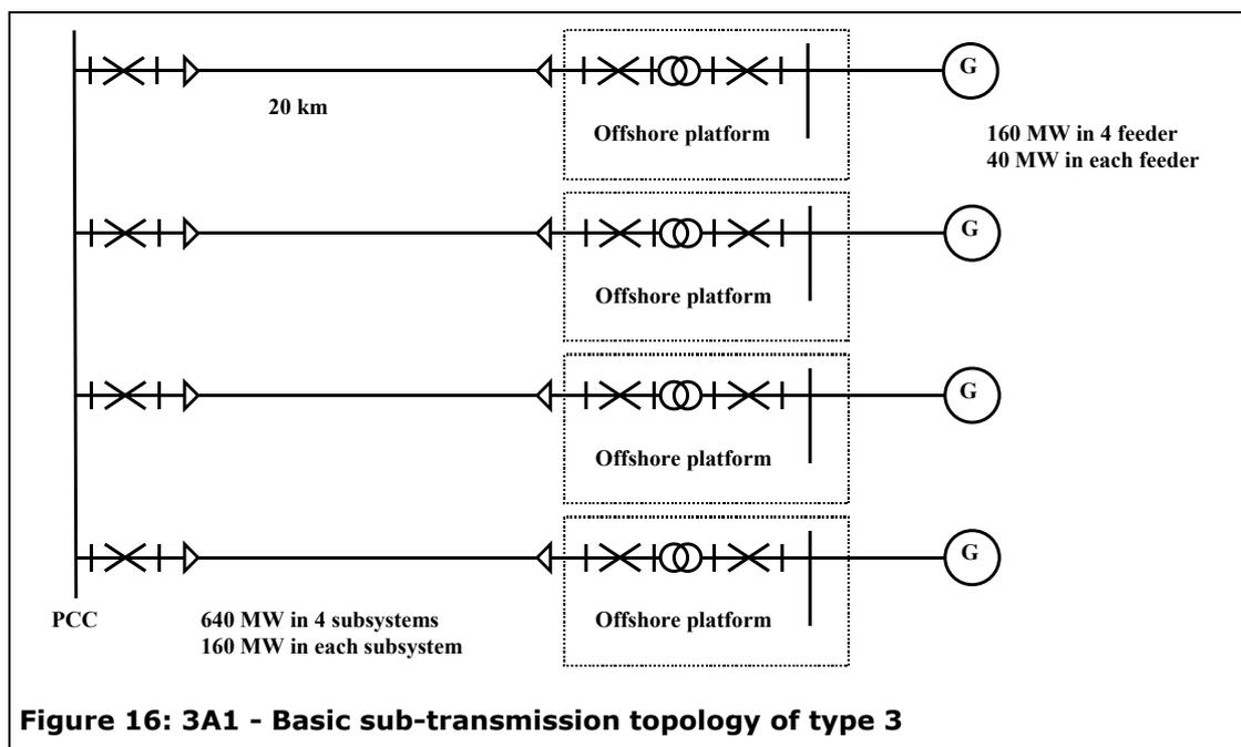
Topology 3A1, where each sub-transmission cable is carrying 160 MW. The study shows that the expected annual energy not supplied is **165.924 GWh** (note: when the whole wind park is studied the expected annual energy not supplied is 330.16 GWh) . The main contribution is from the 150 kV sub-transmission cables.
