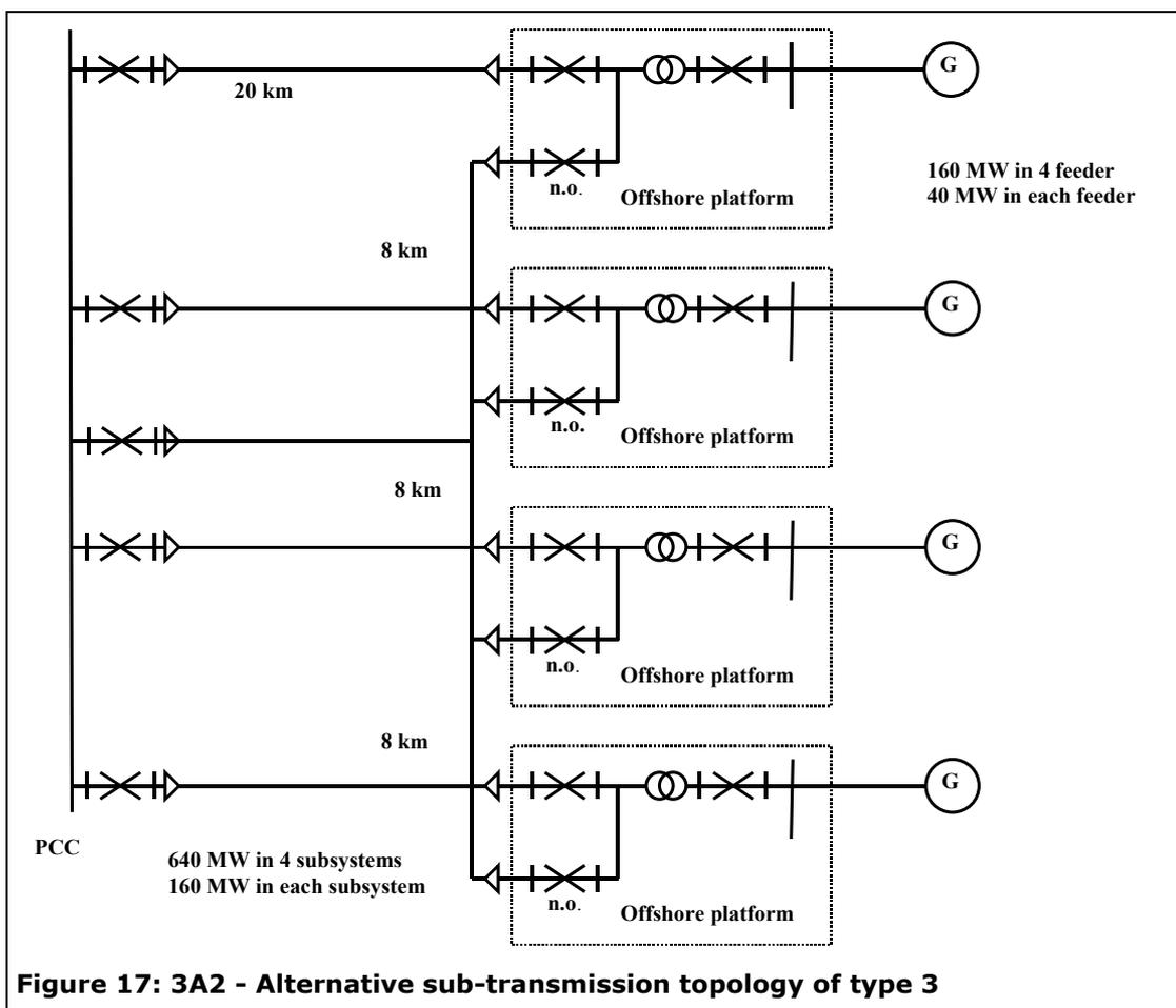
**Figure 17: 3A2 - Alternative sub-transmission topology of type 3**
