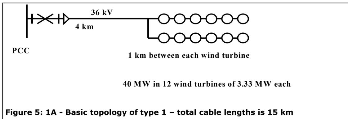
All 12 wind turbines are connected together without load-switches and the feeder cable can transfer 40 MW. The study shows that the expected annual energy not supplied is **10.362 GWh** (annual energy supplied at rated generation is 350 GWh). The contribution is of course from the cables. As the feeder cable is much longer than each of the interconnecting cables, high contribution comes from the feeder cable.
