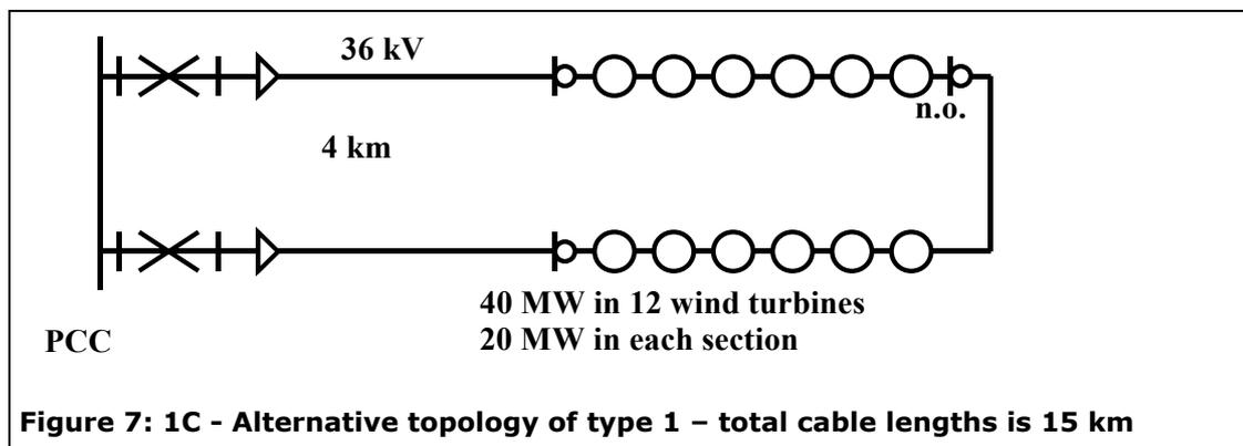
Alternative topology 1C, with load-switches installed in some wind turbines. The redundancy consist of an additional feeder cable, an additional switchgear in the PCC, five wind turbine-placed load-switches and control system. The expected annual energy not supplied is **5.526 GWh** (350 GWh). The contribution from the interconnecting cables is still high.
