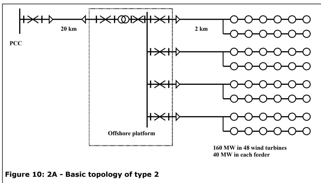
Each feeder is capable to transfer 40 MW and the sub-transmission cable can transfer 160 MW. The study shows that the expected annual energy not supplied is **82.540 GWh** (annual energy supplied at rated generation is 1400 GWh). The main contribution is from the 150 kV sub-transmission cable.
