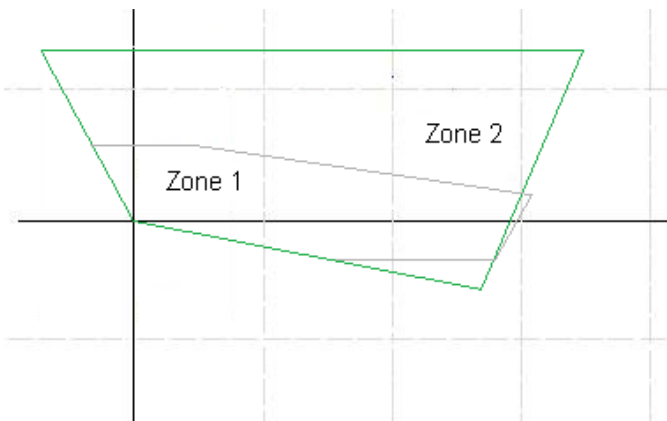
Fig. 12. Adjustment Zones of a distance relay, which illustrates the inclination to Zone 1, because the impedance fault.
