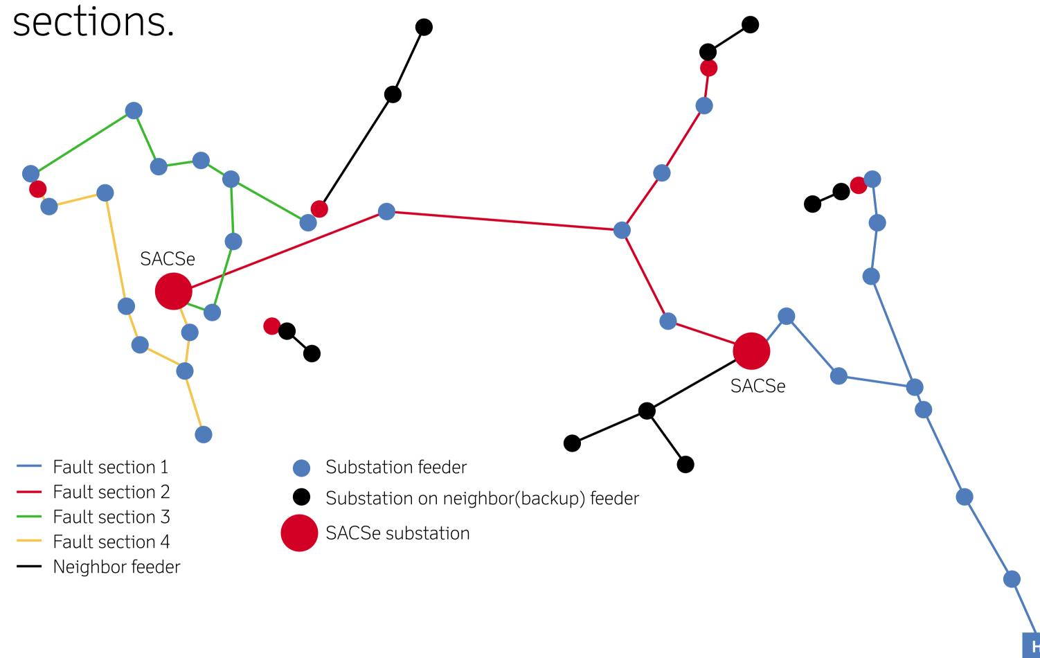
SACSe switching with 2 substations on a feeder with a the fault downstream.
