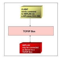
NEPLAN can be connected as Server to a TCP/IP bus. All NEPLAN data and calculation functions can be controlled by a client program. The calculation results will be transmitted over TCP/IP to the database
