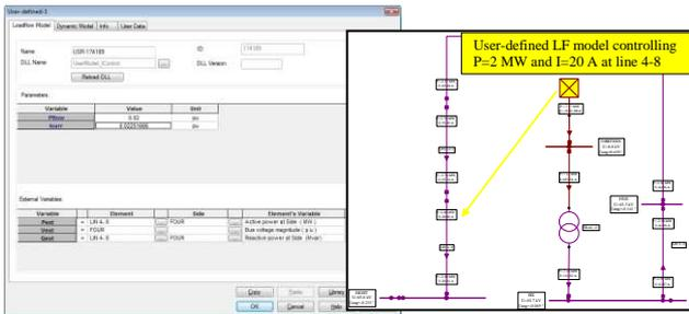
1) **Load flow models** may be defined with the NEPLAN® C/C++ API. Basically the load flow equations will be written in a C/C++ program. The compiled DLL file will then be assigned in the NEPLAN graphical editor. The dialog in NEPLAN show the parameters and signals which have to be defined for the model.
